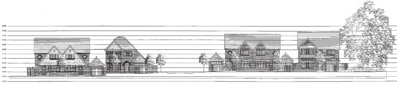
Street Scene C-C Elev 1 FFL 2.00m Elev 2 FFL 2.40m Elev 3 FFL 2.80m Elev 4 FFL 3.20m Elev 5 FFL 3.60m Elev 6 FFL 4.00m
